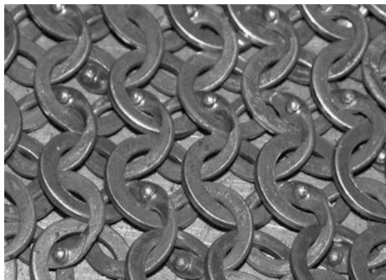
1. Reproduction mail made from 0.050" (1.27mm) pure iron wire. (Photo courtesy of the author)
