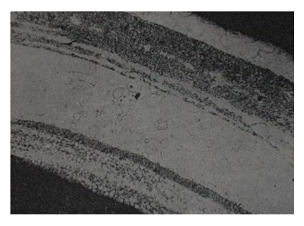
X 100. The heterogeneous nature of the steel from which the wire was drawn is apparent from the banding in the link.
