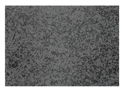
X 2000. Tempered martensite, showing a mass of tiny carbide particles
