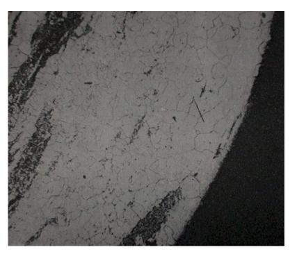
X 100 Mostly ferrite with streaks of a dark-etching material.
